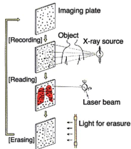
The BaFX: Eu<sup>2+</sup> (X = Cl, Br or I) crystal is an ionic crystal having a tetragonal structure, and Ba is replaced with the Eu<sup>2+</sup> ion to create a solid solution. This crystal, when irradiated by radiation, for example, produces mainly two types of color centers in the crystal where an electron is trapped in an empty lattice of the F or X ion. The color center actually produced mainly depends on the discrepancy between the stoichiometric composition of F and X. The
