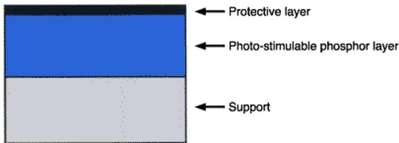
Exposure of samples to the Imaging Plate is performed in a manner similar to that of photo-film. The exposed Imaging Plate is scanned with a laser beam of red light while the plate is being conveyed with high accuracy in a phosphor reader as shown in Figure 2.
