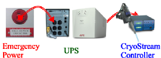
Figure 6 Emergency + UPS Power for CryoController
