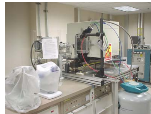
R-Axis IIc IP detector w/ Blue Osmic confocal Max-Flux mirror system (Rigaku/MS)
