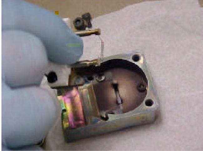
**Figure 8** Replacing a new x-ray filament in side the cathode assembly
