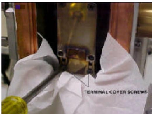
*Figure 4 Cathode assembly with Kim Wipes placed beneath the assembly*
