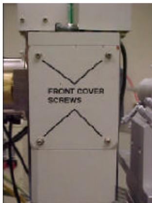
*Figure 2 Front vacuum cover assembly with screws highlighted*
