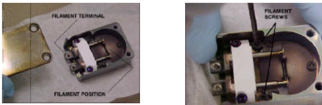
**Figure 7** a) Removing the back cover reveals the filament. b) Removing the screws to remove burnt filament
