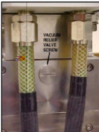
*Figure 1 Vacuum release knob located beneath the rotating anode chamber*
