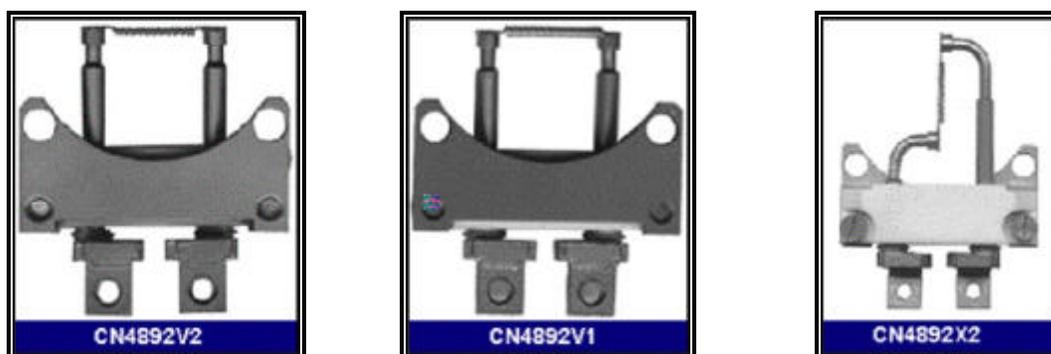
**Figure 9** New Rigaku filaments: CN4892V2 fine focus ( $0.3 \times 3.0 \text{ mm}^2$ ) CN4892V1 fine focus ( $0.5 \times 1.0 \text{ mm}^2$ ) & CN4892X2 line focus ( $0.2 \times 0.2 \text{ mm}^2$ ).
